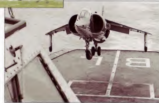
Below: The Harrier proved the concept of using high-performance jets at sea without the need for conventional aircraft-carriers. Here an early Harrier uses its vectored thrust to make a vertical landing on the helicopter cruiser HMS Blake.
